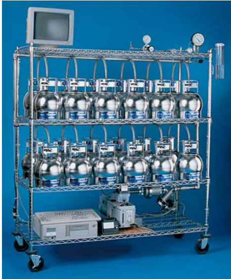
Figure 8 User-designed system for cleaning 24 six-liter canisters.
